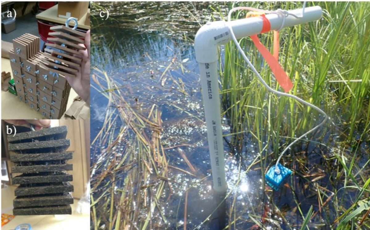
Fig. 3. Hester-Dendy samplers are artificial substrate samplers that are deployed in water and given time to allow macroinvertebrates to colonize the plates: a) Hester-Dendy samplers prior to deployment, b) Hester-Dendy sampler after being deployed one month in submergent plant community with colonized macroinvertebrates, c) sampling apparatus used to anchor and suspend Hester-Dendy samplers in the meadow at Munuscong Bay in 2020.
